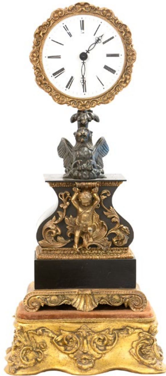
24. Robert-Houdin "La Fleur Mysterieuse" Mystery Clock. Paris, ca. 1830s. A "series one" mystery clock with concealed mechanism. Enamel dial and steel minute and hour hands, roman numeral hour markers and minute bits. Time and strike to train movement. Patinated griffin with foliage support concealing the clockworks that operate the hands. Rear of the base inscribed "Brevet D'invention." The clock resting on a separate base with hollow center allowing the pendulum to swing. 7 x 4 ¼ x 2 ¾". With key. Detailed condition report available upon request; third party shipping required.
